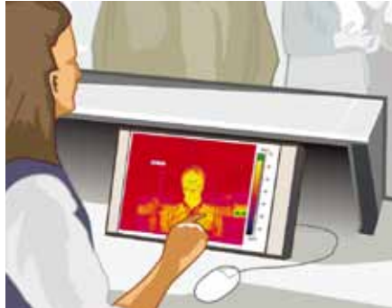
Step 2: IR camera operator looks at a color monitor that shows audible and/or visible color alarms when an individual shows an "out of norm" body temperature.
